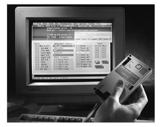
overlay memory. Integrated support for Real-Time Operating System kernels provides visibility of target/OS interactions. An interval timer provides statistical measurements of code, and external triggering capability supports logic state analysis. Manufacturing or field testing is supported with powerful macros, clip-on adapter support, standalone mode, and portable communications.
